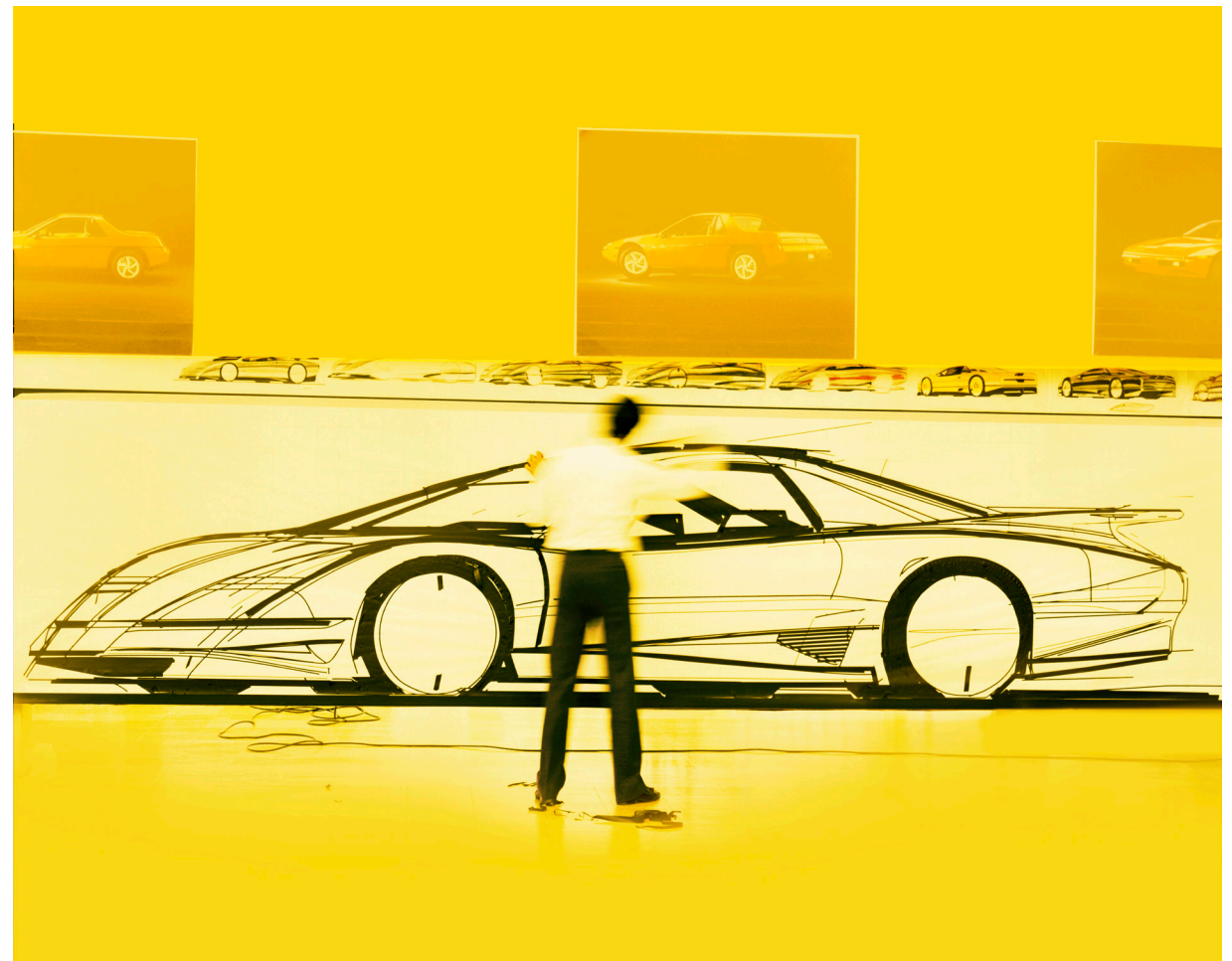
Designer John Cafaro "tape drawing" for the Pontiac F-body program that would result in the Pontiac Firebird, ca. 1984
